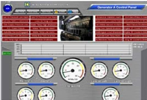
While the main purpose of the power monitoring system is to improve reliability and response time, it also provides automated monthly ATS and Gen Set testing and all the EPSS testing documentation needed to fulfill the requirements of the Joint Commission Environment of Care Standard EC.2.14. and NFPA 99 and 110. These once time-consuming and labor-intensive requirements can now be easily automated with less labor and a ready-made report created by the system.
